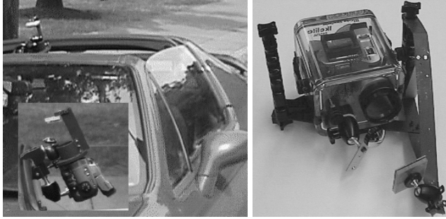
Figure 5: Some custom omni-directional cameras for vehicle and underwater use.
