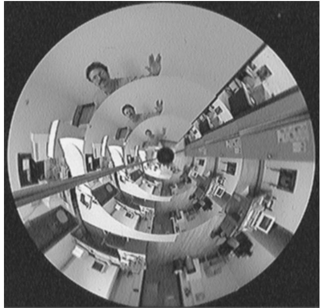
Figure 7: A panoramic pyramid image of size 480x480. The "edges" of the mirrors only distort 1 pixel. (Because of alignment errors in the mounting the smallest mirror is displaced slightly downward.)
