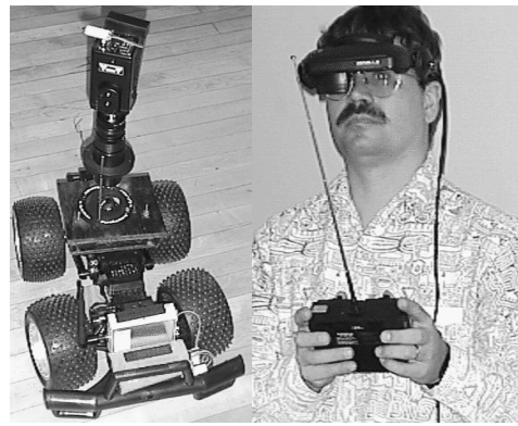
Figure 4: Omni-directional camera on Remote Control Car and Remote Reality Driver.
