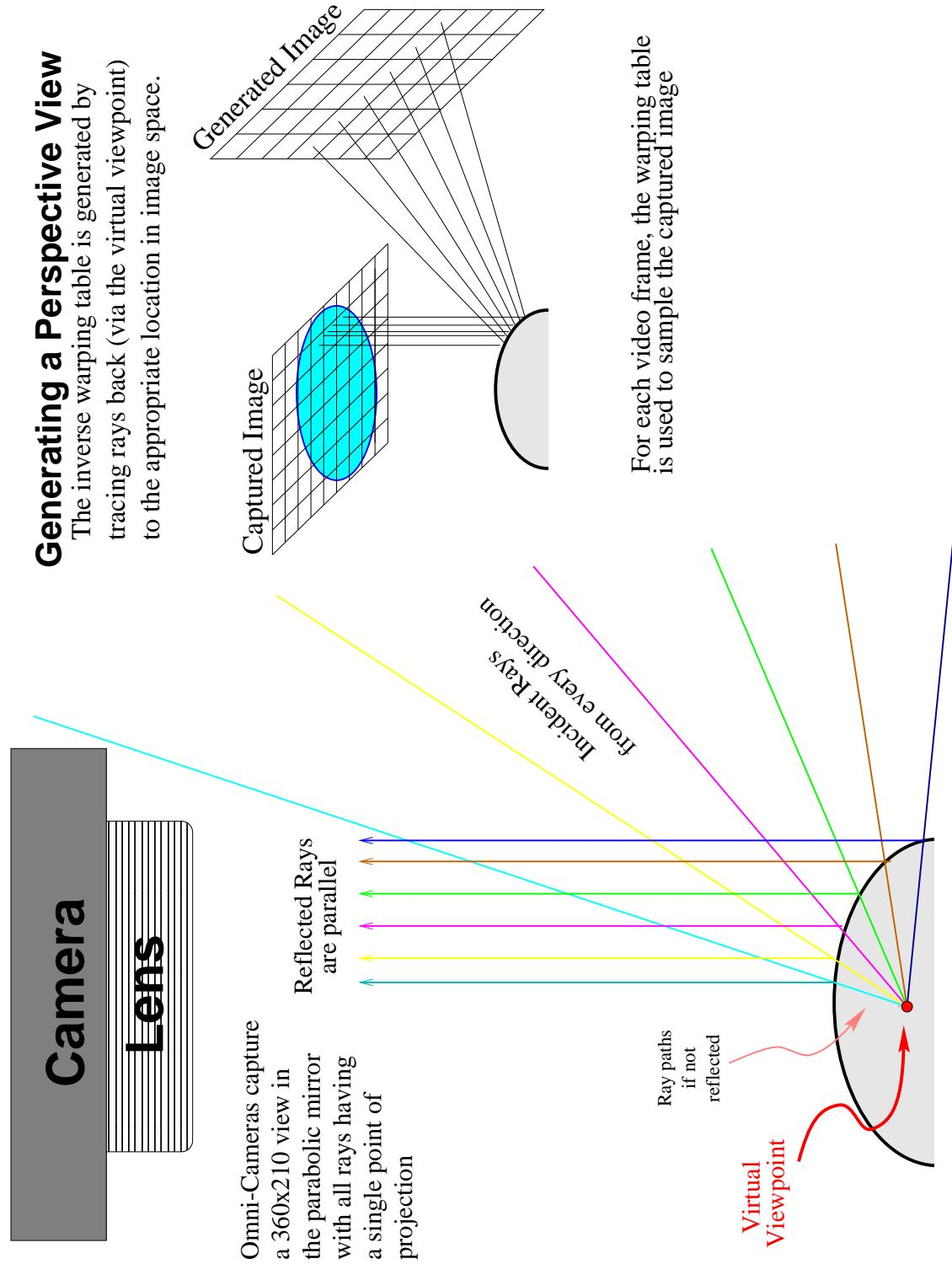
Figure 1: Omni-directional Imaging Geometry
