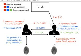
**Fig. 3**. The data-transfer steps for the one-way, two-way, and three-way protocols described in Section 3.2. It is assumed that Alice has Bob's certificate  $C_B$  at the beginning of the one-way protocol.
