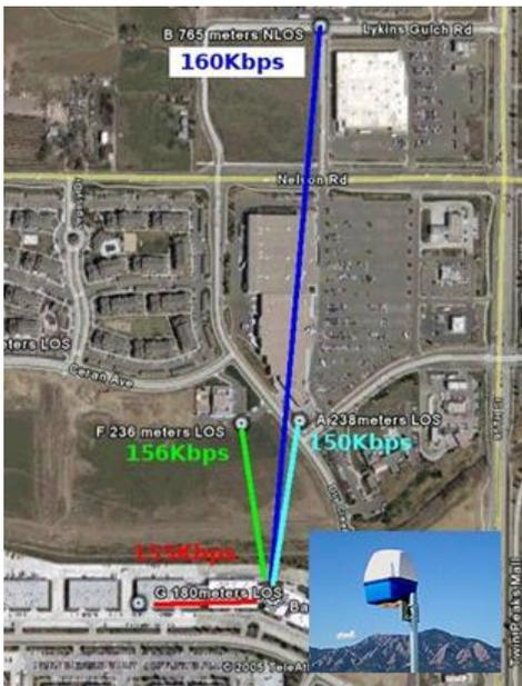
Figure 3 Extended Range ZigBee Connection
