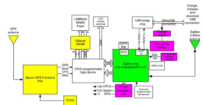
Figure 4 GeoZigBee Device Components
