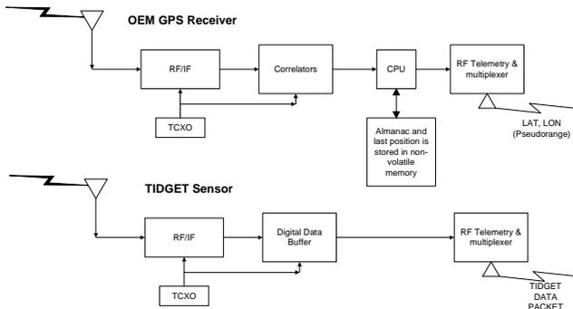
Figure 2 TIDGET Sensor
